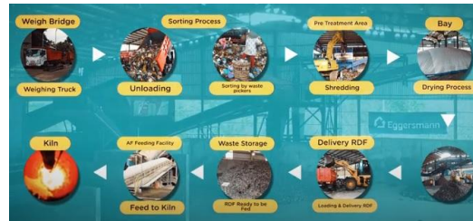
Figure 2. RDF process flow
